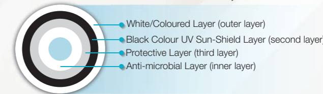
Cross-section of 'Vectus Safe 4 Layer' water tank
