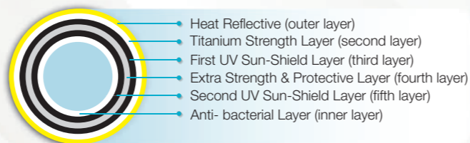
Cross-section of 'Vectus T-90' water tank
