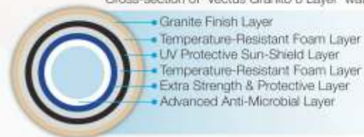
Cross-section of 'Vectus Granito 6 Layer' water tank:
