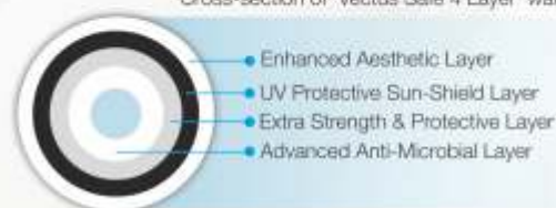
Cross-section of 'Vectus Safe 4 Layer' water tank
