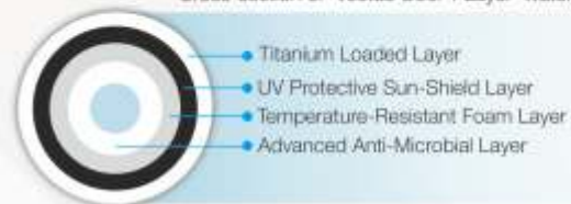
Cross-section of 'Vectus Cool 4 Layer' water tank
