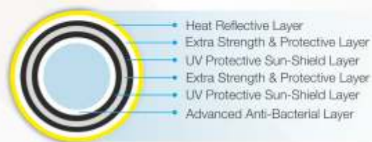
Cross-section of 'Vectus T-90' water tank
