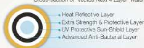
Cross-section of 'Vectus Next 4 Layer' water tank
