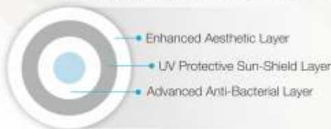
Cross-section of 'Vectus Silk 3 Layer' water tank
