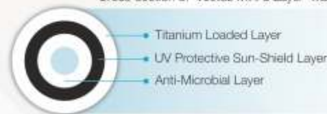
Cross-section of 'Vectus Mini 3 Layer' water tank
