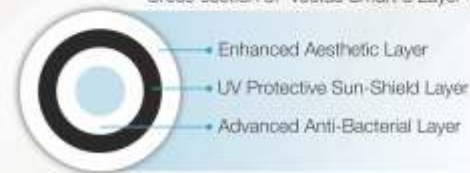
Cross-section of "Vectus Smart 3 Layer" water tank
