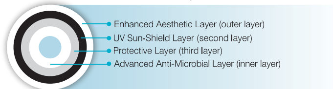
Cross-section of 'Ganga Health 4 Layer' water tank
