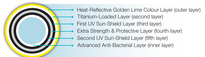
Cross-section of 'Ganga T-90' Water tank
