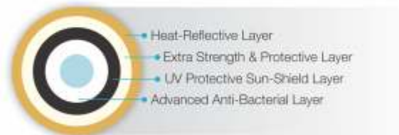
Cross-section of 'Waterwell Wonder 4 Layer' water tank
