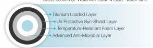
Cross-section of 'Waterwell Italian 4 Layer' water tank
