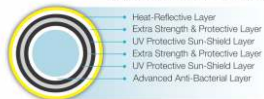
Cross-section of 'Waterwell T-90' water tank
