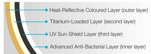
Cross-section of 'Waterwell Wonder 4 Layer' water tank
