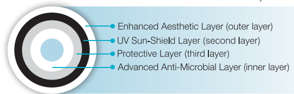
Cross-section of 'Waterwell Health 4 Layer' water tank
