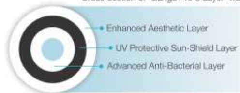
Cross-section of 'Ganga Pro 3 Layer' water tank
