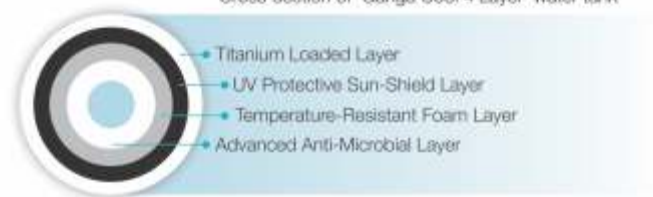
Cross-section of 'Ganga Cool 4 Layer' water tank
