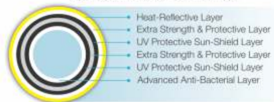
Cross-section of 'Ganga T-90' Water tank
